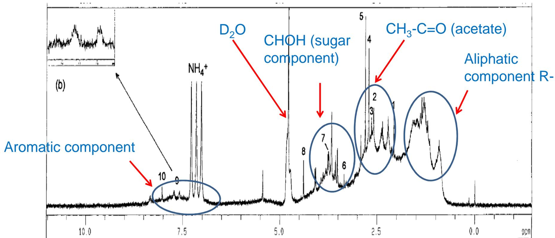
NMR spectra of fine particles 0,62-1,1  $\mu\text{m}$
